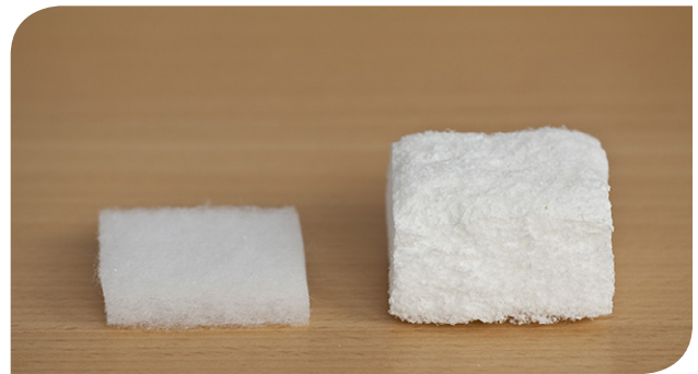
Picture 3. Photo of impregnated nonwoven before and after the expansion of Expancel.
